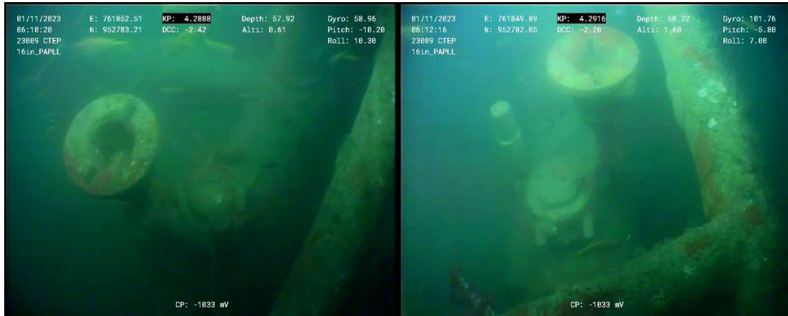
Figure 15 – PAPLJ-Y2-16" PAPLL branch: Ball Valve - VB6 Indicator obscured
