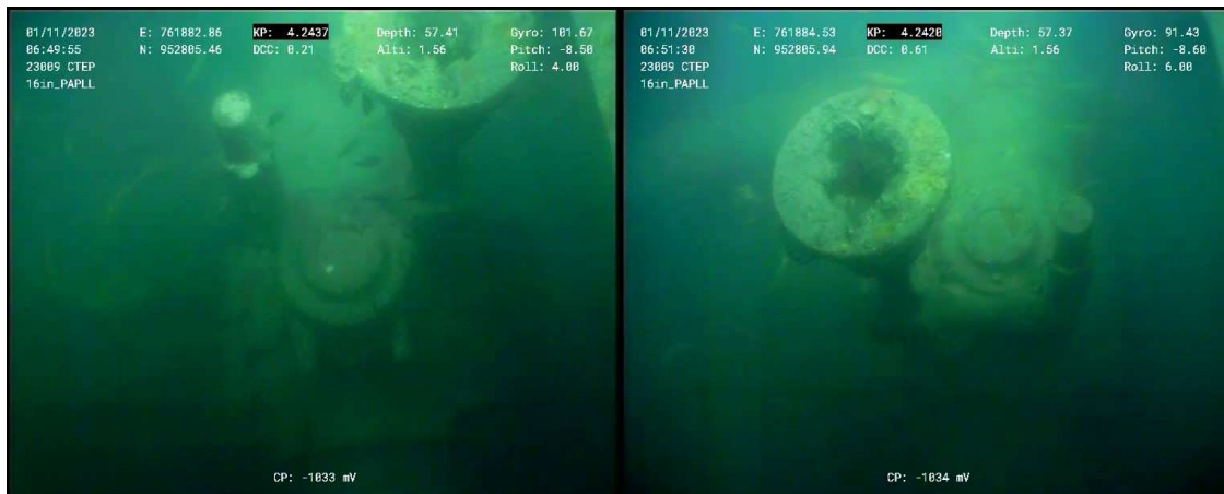
Figure 8 – PAPLL-Y1-16" PAPLL branch: Ball Valve - VB4 Indicator obscured
